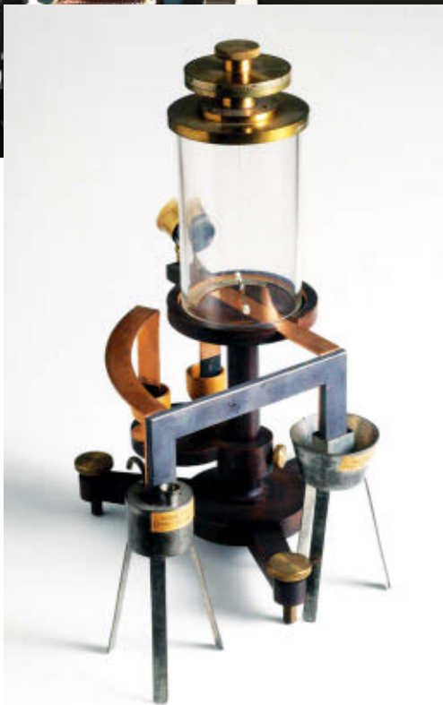
Figure 2. A reproduction of Ohm’s experimental apparatus. The thermoelectric generator in the foreground used a copper and bismuth thermocouple activated with boiling water and snow. The torsion balance consisted of a magnetized needle positioned directly over and parallel to a copper strip connected to a test conductor, the ends of which attached via the two small mercury-filled cups in the far background. ©The Board of Trustees of the Science Museum (London). Creative Commons BY-NC-SA 4.0.
