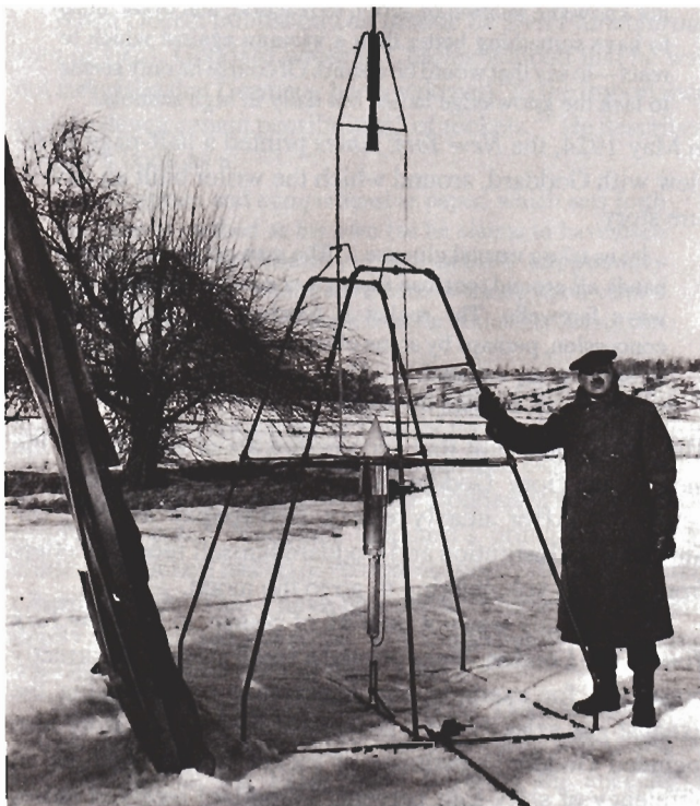
Fig. 3. Robert H. Goddard posing with the first successful liquid-fuel rocket prior to its secret launch on March 16, 1926. Goddard did not notify his financial backers of the successful flight until May 5, 1926. For this rocket, fuel was delivered to the nozzle (positioned at the top) via pressurized tanks. No pumps were used. Photograph courtesy of Goddard Collection, Clark University.
