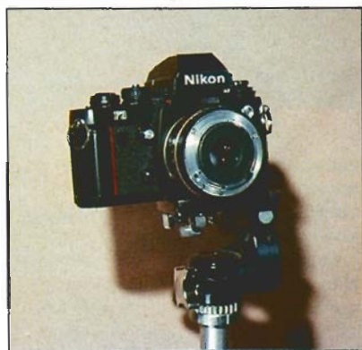
A 50mm lens mounted backwards on a Nikon F3 using an inexpensive reversal ring.
