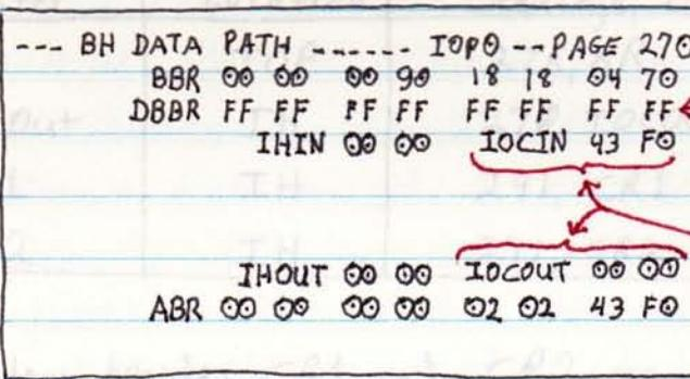
Delayed BBR → allows holding BBR for one cycle before storing into BH RAM on a write operation.
