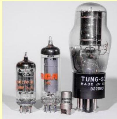
Figure 2—Size comparison of ordinary tubes to a Nuvistor (second from right)
