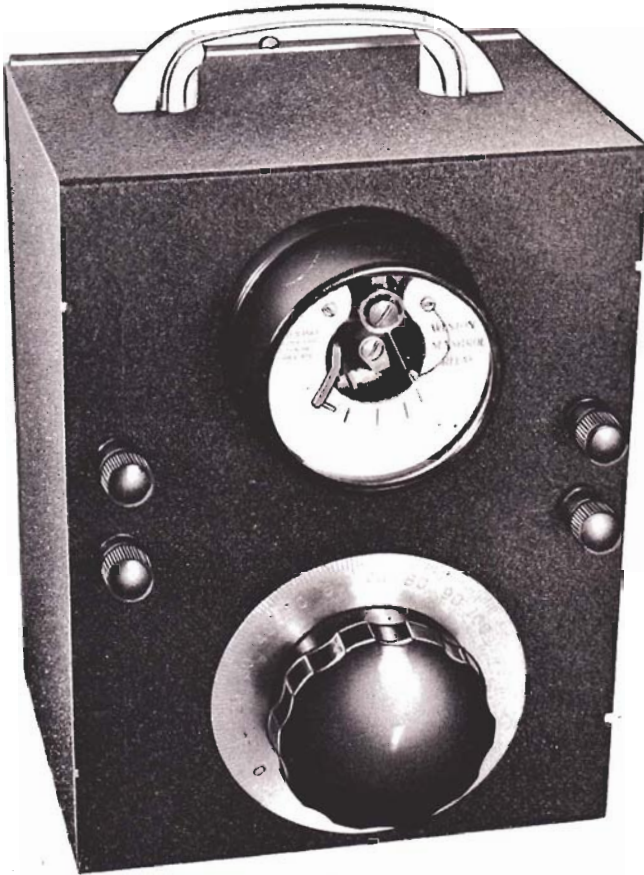
Figure 25. Front View of the Radio-Controlled Relay.
