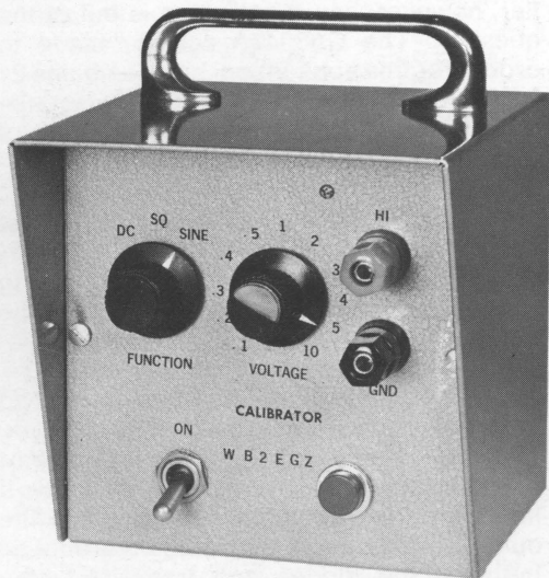
Figure 1: Exterior view of three-mode voltage calibrator constructed by WB2EGZ. A rather sophisticated circuit has been compressed into a 5-by-5-by-5-inch "cowl box."
