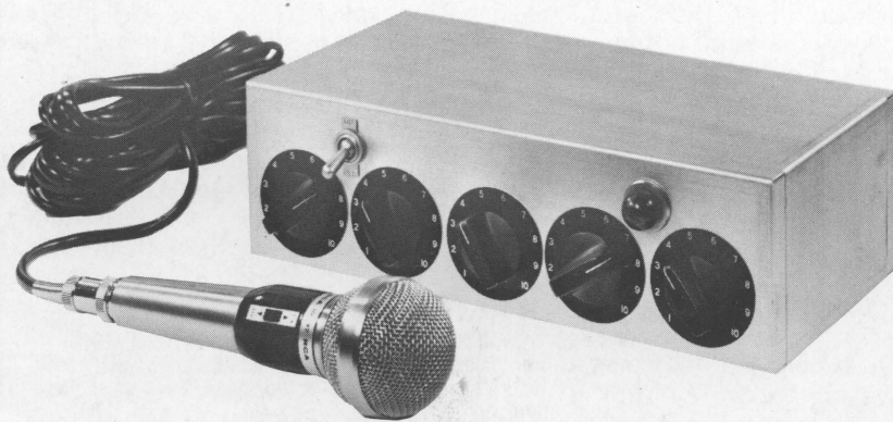
Figure 1: Exterior view of assembled audio control system for SSB, consisting of a microphone preamplifier, audio oscillator, and an audio mixer, compressor, and line driver.
