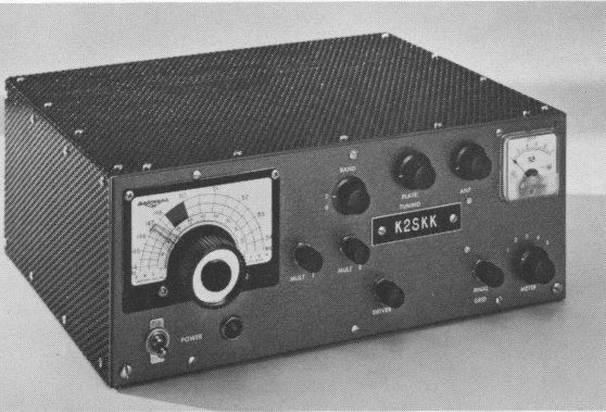
Front view of WA2ELL's and K2SKK's mobile 50-watt transmitter. Unit measures approximately 12 inches in width, 5 inches in height, and 10 inches in depth.
