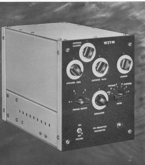
Front view of W2YM's 120-watt 50-megacycle transmitter. [Note the air-intake holes on the side of the blower (or bottom) chassis. They each measure \frac{3}{8} inch in diameter.]
