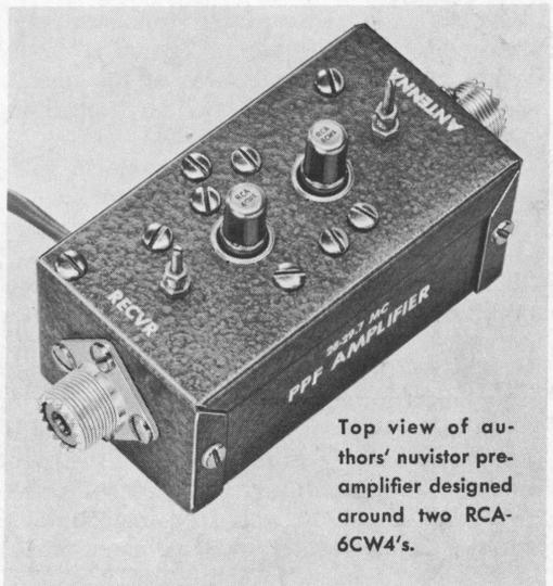
Top view of authors' nuvistor preamplifier designed around two RCA-6CW4's.
