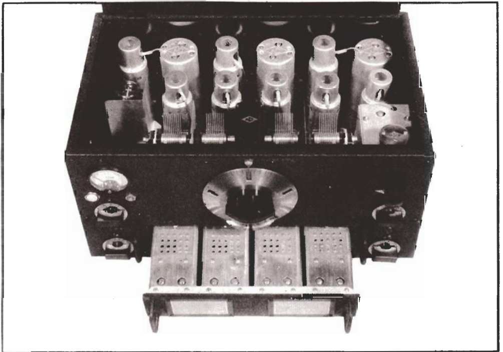
The front of the HRO, with a coil unit partly removed. By changing connections on the terminal plate of each coil in the unit, band-spread or general-coverage tuning can be obtained. This is one of the features that makes the receiver adaptable to a wide range of service
