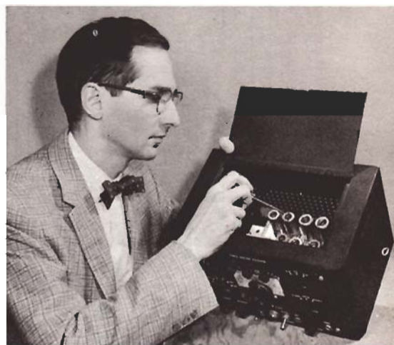
K2LMG DISPLAYS his 20-watt, 14-tube, 144-megacycle SSB exciter. Dave is a consulting engineer in the Advanced Radar and ECM Engineering group at General Electric's Advanced Electronics Center at Cornell University, Ithaca, New York. He has been with General Electric for 13 years and has participated in developing a number of advanced electronics, radar and weapons control systems. He is the author of articles in QST on measuring VHF station performance, and measuring antenna patterns using the sun. K2LMG since 1957, Dave is a senior member of IRE.
