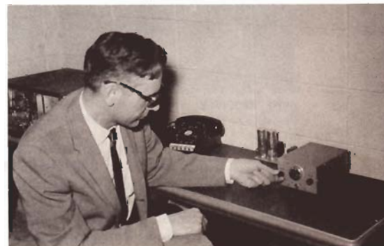
COMPLETE VHF RECEIVER and companion power supply for AC operation. Borg Microdial was used on this model for tuning.
