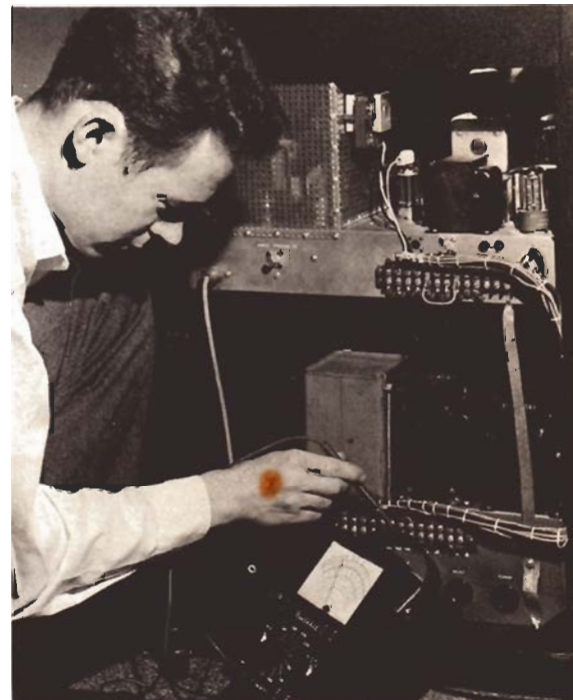
REAR VIEW of transmitter at W7KCS/9, with complete power supplies and modulator in lower unit, and RF exciter and power amplifier, and audio preamplifier in upper unit.
