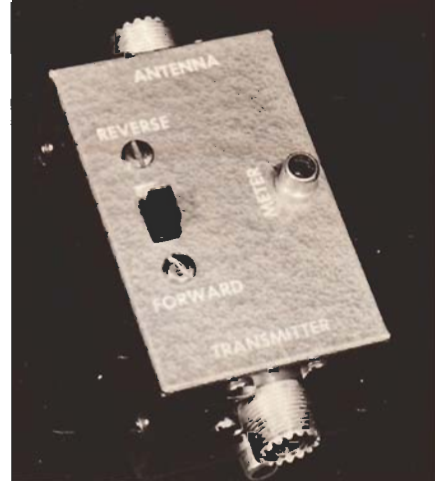
TOP VIEW of the RF pickup unit. Compact size and complete shielding contribute to maintaining 50-ohm impedance through unit, minimizing disturbance in line. Box size is 3¼ x 2½ x 1⅝ inches.
