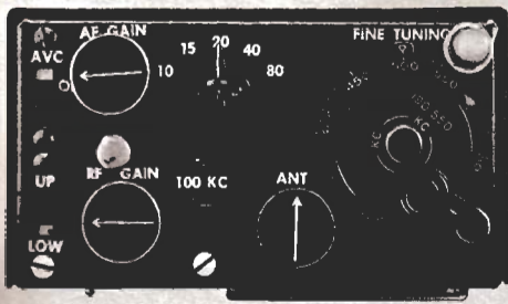
PANEL VIEW PHOTO of the bandswitching converter. Only the controls marked "RF GAIN," "ANT.," and "80-40-20-15-10" (the bandswitch) actually control circuits in the converter.
