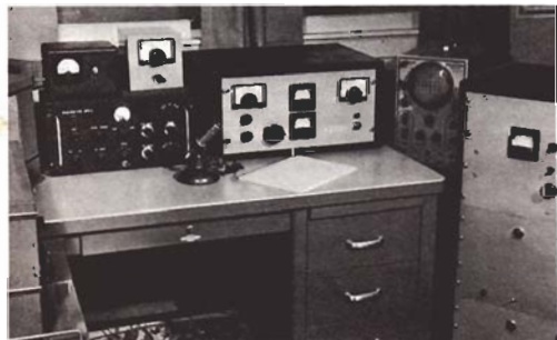
MONITOR-ADAPTED 'SCOPE AT K2IOW, at right of desk, a Heath type O-5 constructed from a kit. Space for the adapter components and additional panel controls can be found in most test type oscilloscopes.
