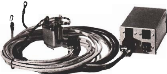
Fig. 10. View of the suggested low-voltage cable harness, main power relay, RY_3 , and the control box wired according to Fig. 11 below.
