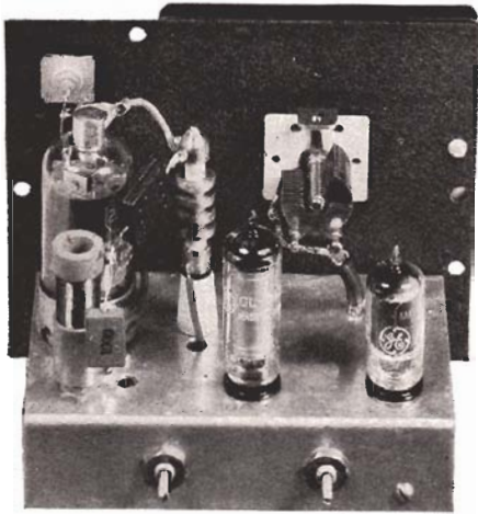
Fig. 5. Back view of the E-P Rig. Coils L_1 (right) and L_2 (left) are tuned through holes in the cabinet rear plate. The GL-2E26 plate coil, L_3 , mounts directly behind this tube.
