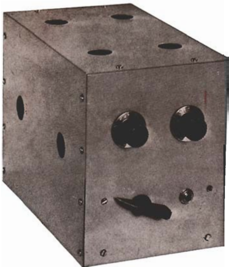
Fig. 6. Front panel view of 6-Meter CD Receiver. ANL control at upper left, gain control at upper right.
