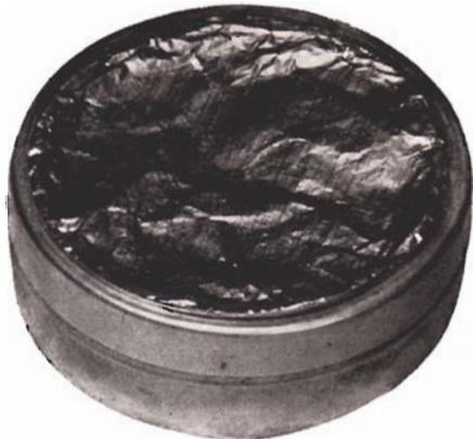
Fig. 1. View of Electrophone showing aluminum foil diaphragm
