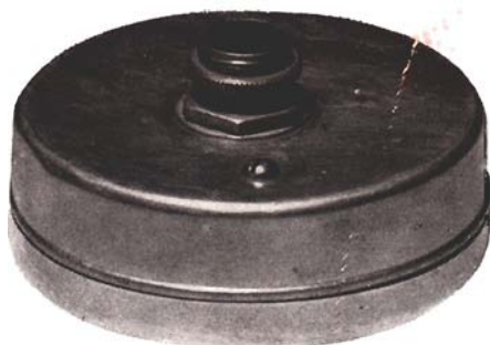
Fig. 6. Rear view of Electrophone showing microphone connector
