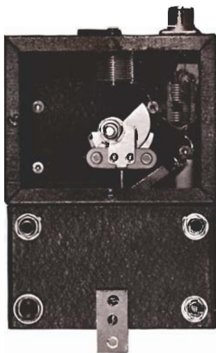
Fig. 3. Front Panel View of MHE Transmitter with Panel of Top Portion Removed
