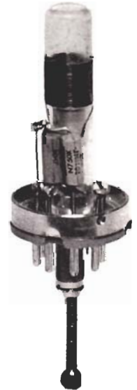
Fig. 3. Detail View of Oscillator Plate Coil.
