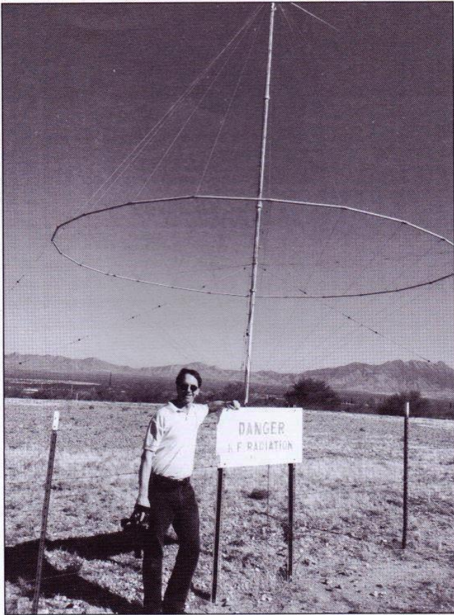
Figure 2—The sign by the 80-foot tall discone antenna reads, “DANGER: RF RADIATION” but that certainly wouldn’t apply to N4TRB’s 5-watt QRP signal. On the other hand, it does start one thinking about a mobile kilowatt!
